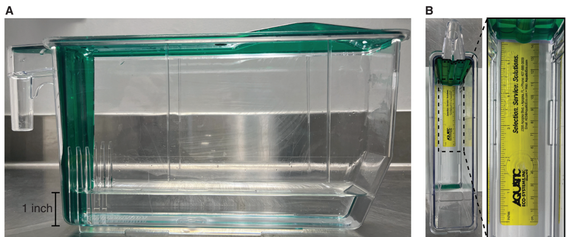
FIGURE 2. Adult tank housing for life span assessment. (A) Complete 1.8-L tank with lid and baffle with ~1 inch of aquatic system water. (B) Photography station for measuring fish at 4 wk of age. Tank is placed above a flat ruler such that the ruler is imaged through the ~1 inch of system water.
